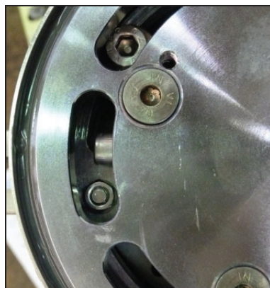
Fig. 17: Alignment of stop screw
