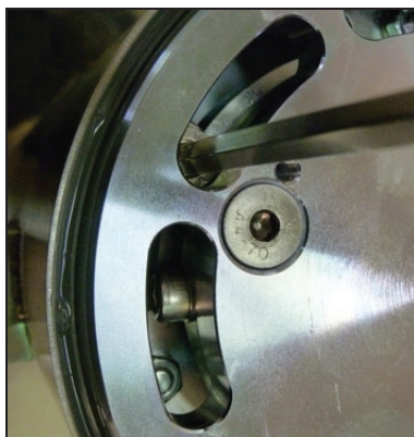
Fig. 19: Adjusting the left end stop
