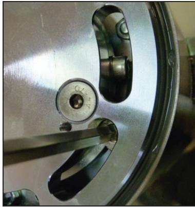
Fig. 18: Adjusting the right end stop
