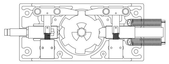
An internal view of an electronically controlled two way 6500 series control head.
