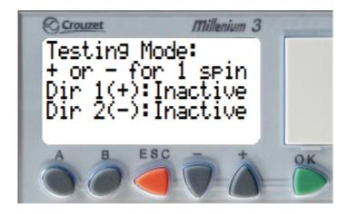
Testing mode simulates valid access control inputs based on the settings defined on the other menu screens. The unit should unlock for the duration of the directional timer or until the unit is rotated. If the button is pressed twice, it should allow two rotations or time out based on the mult-swipe setting. If the button is held and the one shot timers are disabled, the unit will continue to remain open until the button is released and another rotation or timeout occurs.
