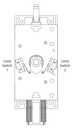
Turnstile control heads use a triangular shaped limit switch cam. One point of the triangle needs to be facing the index pin (bar with two springs) when the cam is in the home position. The two indents in the sides of the triangle are for jigging purposes. It does not matter which point is facing to the springs.
