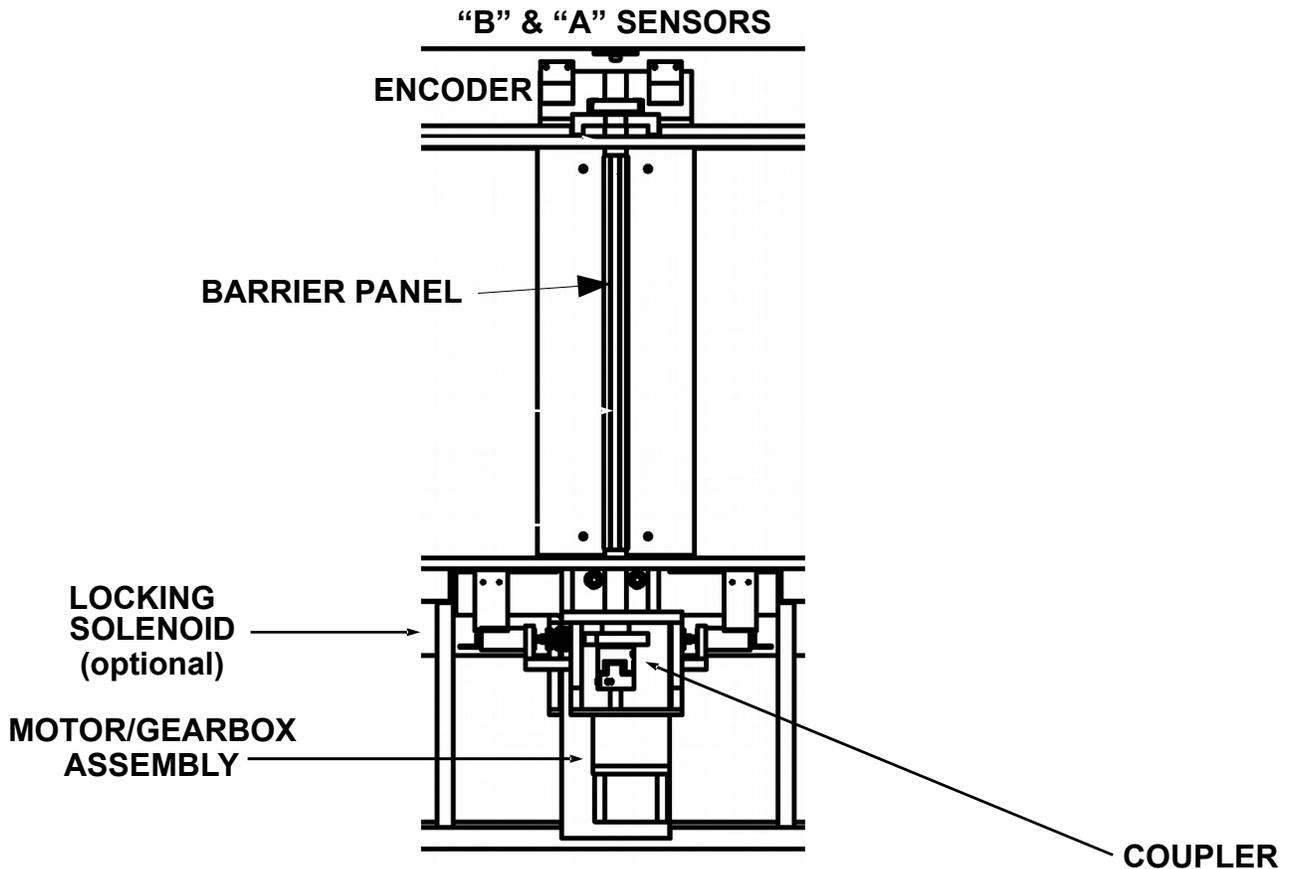
The **Motor/Barrier Assembly** is the center section of the bollard, located between the two pedestals.
